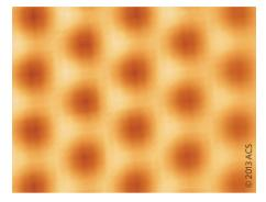
Graphene has a variety of intriguing properties because of its honeycomb lattice. Other materials with such two-dimensional structures are known including hexagonal boron nitride and silicene. However, these materials, like graphene, are typically made of *p*-block elements. Yeliang Wang, Shengbai Zhang, Hong-Jun Gao and colleagues have now shown that twodimensional honeycomb lattice structures can also be created using transition metal atoms.
